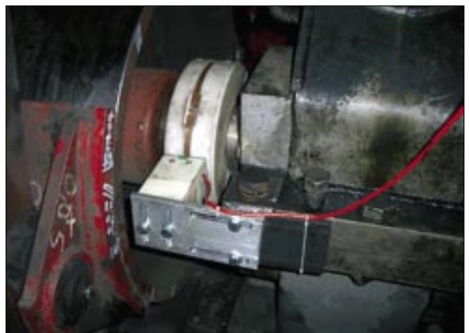
Fig. 1: Inductive torque measurement location
